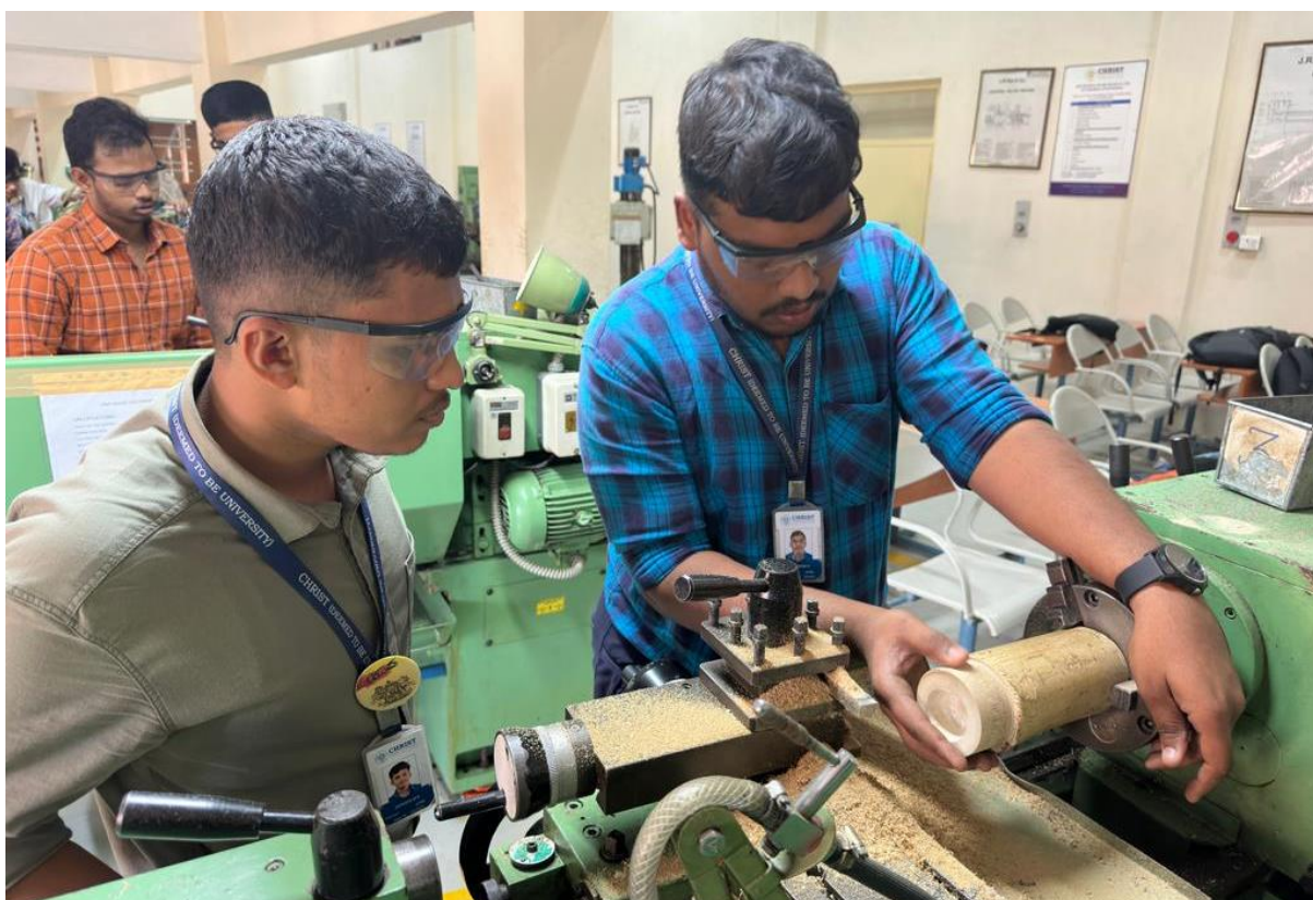
Figure.4 Turning of Bamboo bar by students
